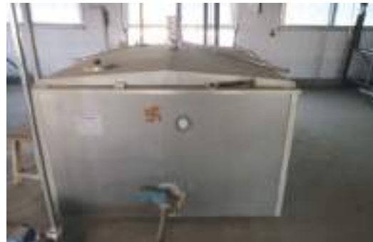
Fig. 3.5: A milk chilling tank of 1000 litre capacity
