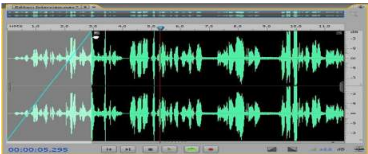
Figure 10: Drag the Fade In handle to the right to create a fade at the beginning of the clip.
