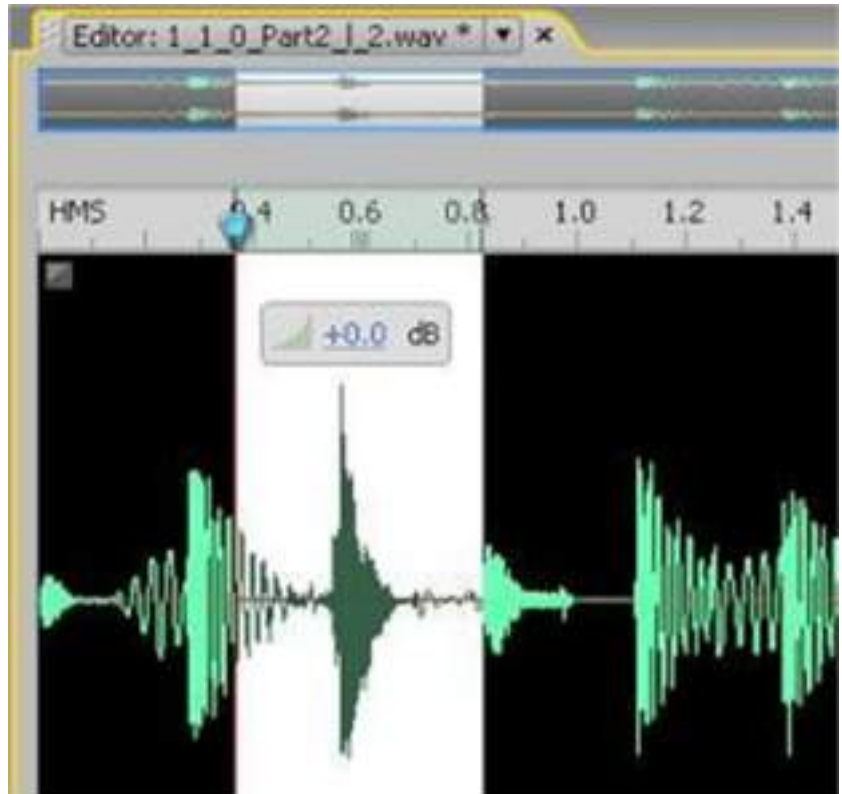
Figure 10: Increase or decrease the amplitude of a range by using the volume pop-up menu.
