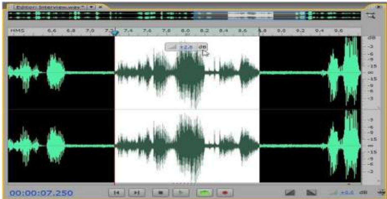
Figure 8: Drag the underlined numbers in the Volume pop-up bubble to change the volume of the selected range
