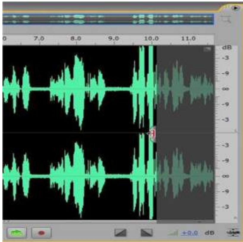
Figure 12: Drag the trim handles inward to trim the beginning and end of clips
