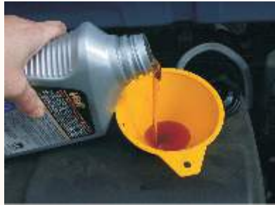
Fig: Fill up oil with funnel
