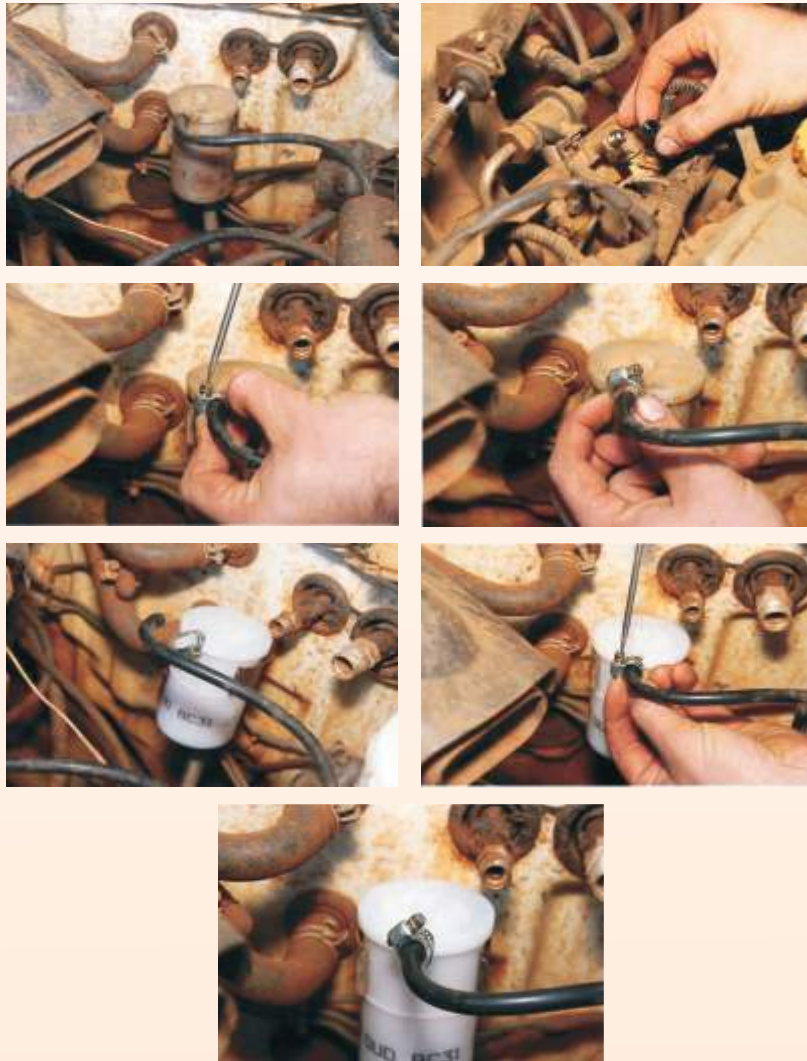
Fig: Photographs of Replacing Fuel Filter
