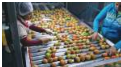
Figure 5.44. Fruit Roller Sorter
