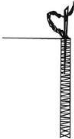
Figure 5. A seam end can be secured by burying it inside the seam.
