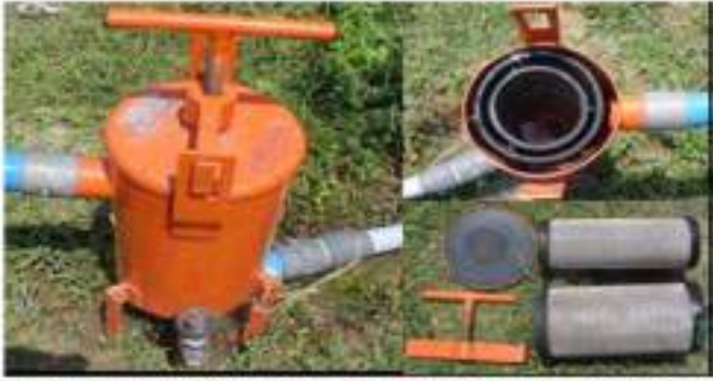
Fig.5.3 Screen filter showing steel wire mesh strainers
