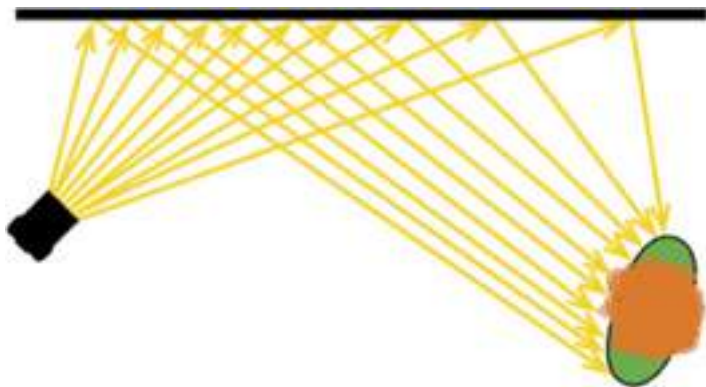
Figure 1.6. Light that bounces off a surface, like a white wall or ceiling, will also come at the subject from many angles and have soft shadows.
