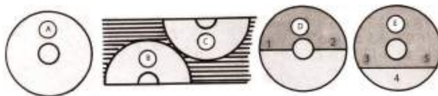
A Without joint, B,C & D With side seam joint, E With joint at circumference
